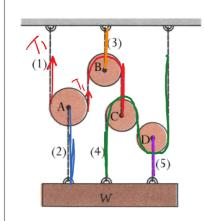
The five ropes can each take 1500 N without breaking. How heavy can *W* be without breaking any?
