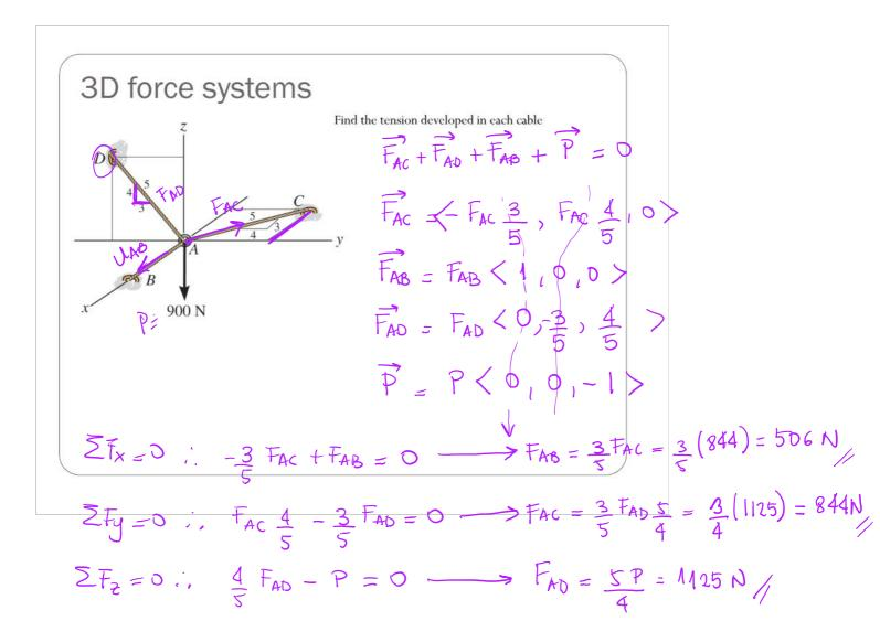
If cable AB is subjected to a tension of 700 N, determine the tension in cables AC and AD and the magnitude of the vector F ra = <0,0,6> m  $r_{B} = \langle 2, 3, 0 \rangle m$ 3 m 1.5 m  $\vec{r}_{c} = \langle -1.5, 2, 0 \rangle m$ 6 m  $\vec{r}_{D} = \langle -3, -6, 0 \rangle m$ JAB = TAB/ITAB/ rab = rb - ra TAC = TC - TA - WAC = TAC/ITAC FAD = FD - FA \_\_\_ (LAD = FAD/ IFAD) FAB + FAC + FAD + F<0,0,1> = 0 FAC UAC + FAD WAD + F<0,0,1>
